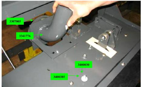
Put (2) WASHER-CONICAL SPRING 3/8 (**3400385**) onto (2) SCR-HEX,3/8-16X1.00 ZP (**3400030**). Place bracket over holes in broom well. Insert bolts in holes through bracket and broom well and center on slotted holes. Put (2) NUT-FLANGE LOCK 3/8-16 (**3400392**) on bolts and tighten.
